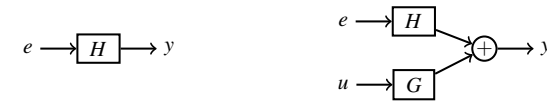
Fig. 2.4: An ARMA system (left) is a deterministic linear time-invariant system with white stochastic process e as an input. An ARMAX system (right) has, in addition, a deterministic input u . The channel e \mapsto y is the “stochastic part” and e \mapsto y is the “deterministic part” of the ARMAX system.
