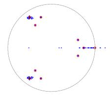
Fig. 2. —true  $\lambda_w$ ,  $\times$ —25 estimates  $\widehat{\lambda}_w$ , obtained with Kung's method. Eigenvalues that are close to the unit circle are more sensitive to additive noisy in the output data. The poorly estimated poles are the ones for  $\lambda_{w,i}=1$ .
