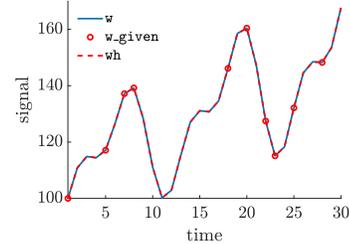
Fig. 1. Reconstruction of a trajectory `w` of a 6th order single-output linear time-invariant system from randomly selected samples `w_given`. The trajectory `wh` reconstructed by the data-driven method matches `w`.
