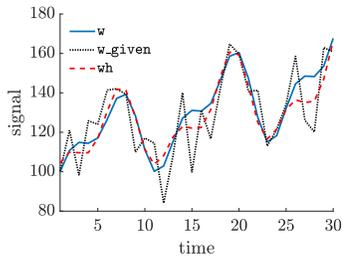
Fig. 3. Smoothing of a noisy trajectory  $w$ . The smoothed trajectory  $wh$  obtained by the data-driven method is an approximation of the true value  $w_0$ . Visually  $wh$  is a better approximation of  $w_0$  than the noisy data  $w$ .
