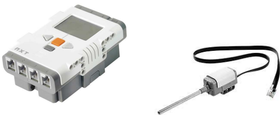
FIGURE 2 The experimental setup consists of the Lego NXT brick (the DSP) and a digital Lego temperature sensor.
