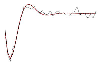
Optimal filtering using identified model  $\widehat{\mathscr{B}}$ , with the 2nd order LTI model class prior
